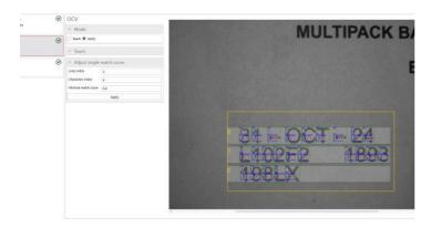
The DCR 1048i OCV can read 1D/2D codes within an application and check the print quality of an imprint (best before date, batch, lot, etc.). No complex set-up with many parameters is required. The sensor only needs to be taught a reference image of the imprint. Faulty prints due to clogged print heads, used ink or adhesion problems can be recognized during the ongoing process. The defective products can be ejected at an early stage.
